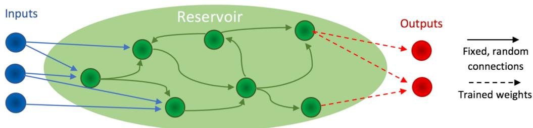
Figure 1. Reservoir computing scheme with random, fixed internal connections and trained readout weights.
