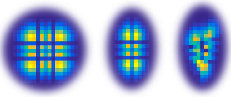
Fig. 4. Visualizations of how the DOE couples a neuron (at the center) to other neurons. Yellow means strong coupling, dark blue means no coupling.
