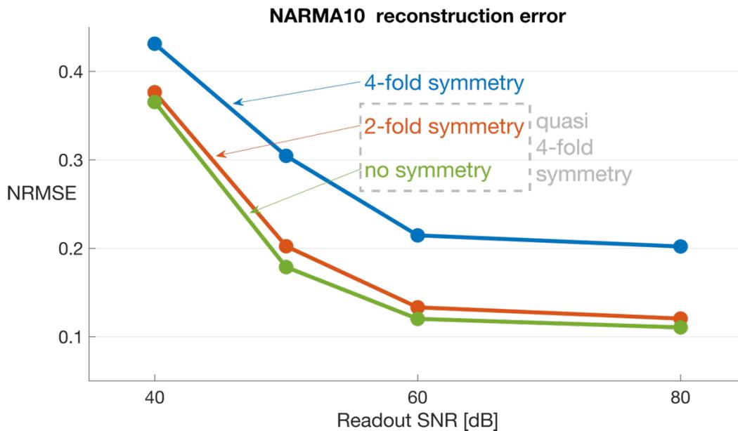
Fig. 5. Simulated RC performance on NARMA10 signal reconstruction task for varying degrees of symmetry of the diffractive coupling scheme, after optimization using simulated annealing. Noise on the output photodiode was simulated and the readout SNRs were calculated w.r.t. the average neural power level. For perfect reconstruction, the Normalized Root Mean Square Error (NRMSE) is 0.
