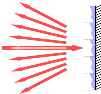
Fig. 3. The DOE's periodic phase profile ensures diffraction under a discrete set of angles.
