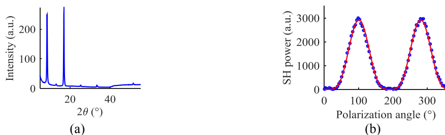
Fig. 3. (a) XRD \theta - 2\theta scan of BNA. (b) Measurement and fit of SH power for normal incidence and varying input polarization ( 0^\circ corresponds to s-polarized light). The PBSC in front of the detector is oriented such that p-polarized SH waves (polarization angle of 90^\circ ) are transmitted.
