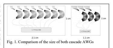
The overall device size of the ultrabroad-spectral-range flat-top cascaded spectrometer is half of that of the conventional one as is shown in Fig 1. The biggest advantages of the proposed spectrometer are the broad-spectral-range operation and the compact device size, which make it very attractive for many different applications. Among these are hand-held OCT, biosensing (smart food packaging), space based astronomy and many more.
