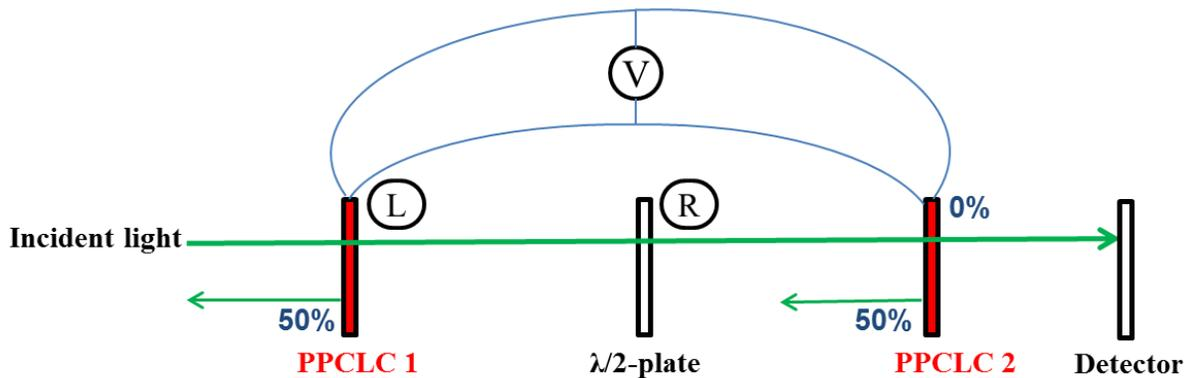
**Fig.1** Schematic drawing of the device operation to modulate unpolarized incident light.
