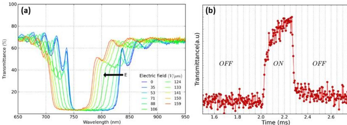
**Fig. 2** a) Transmission spectra for unpolarized light b) Switching of the transmission for light with 850 nm wavelength for a block wave electric field (150 V/ $\mu$ m, 2 kHz) for a full PPCLC- $\lambda/2$ -PPCLC device with two 8  $\mu$ m thick PPCLCs.
