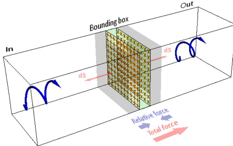
**Fig. 1:** The optical force due to circularly polarized radiation on a bilayer metasurface decomposes into a difference force between individual sheets and a total force in the direction of propagation of the radiation. The bounding box allows calculating the optical forces with the Maxwell stress tensor formalism.
