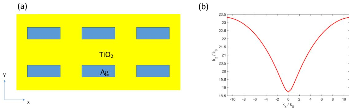
**Fig. 3:** (a) Rectangular nanorods array with nanorods of silver in a  $\text{TiO}_2$  medium. (b) Isofrequency contour in the  $x$ - $z$  plane for a nanorods array with rod of width = 20 nm and height = 10 nm with a periodicity of 30 nm
