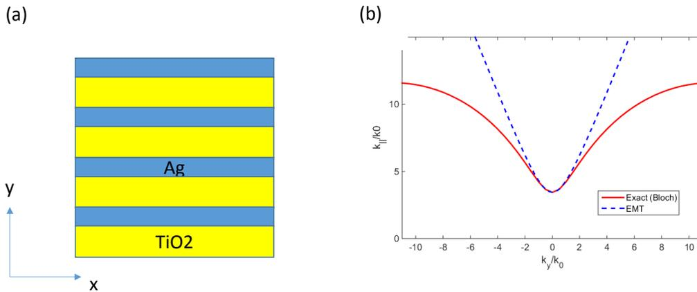
**Fig. 2:** (a) Periodic metal-dielectric multilayer structure with silver as metal and TiO<sub>2</sub> as dielectric. (b) Isofrequency contour at a wavelength of 700 nm for multilayer structure with a metal thickness of 10 nm and a dielectric thickness of 20 nm. Red line is the exact calculation and blue line is the effective medium theory.
