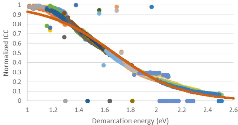
**Fig. 2:** Replot the accelerated aging test result in demarcation energy versus normalized ICC.
